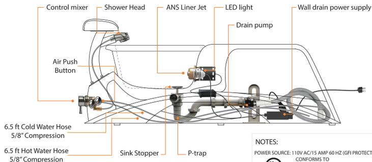
Note: The wall drain system is shown in the above diagram
